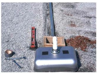
Lysimeters were constructed using stainless steel kitchen sinks (shown here inverted before installation) that collected the putting green leachate and allowed it to be collected in collections bottles at the edge of the greens.
