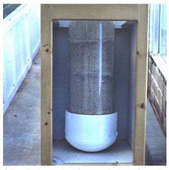
Column like those under turf boxes to simulate golf greens in the greenhouse to determine leaching of nitrate-N and phosphorus.
