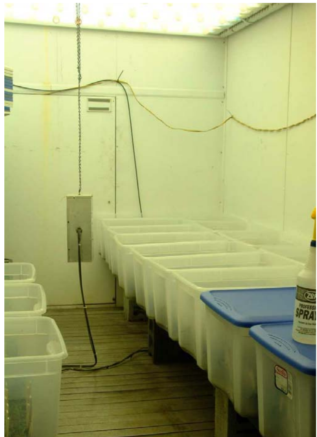
Growth chamber utilized in greenhouse inoculation method 2. Containers with lids were utilized to maintain leaf wetness. The disease response from this technique correlated well with natural field infection of gray leaf spot.
