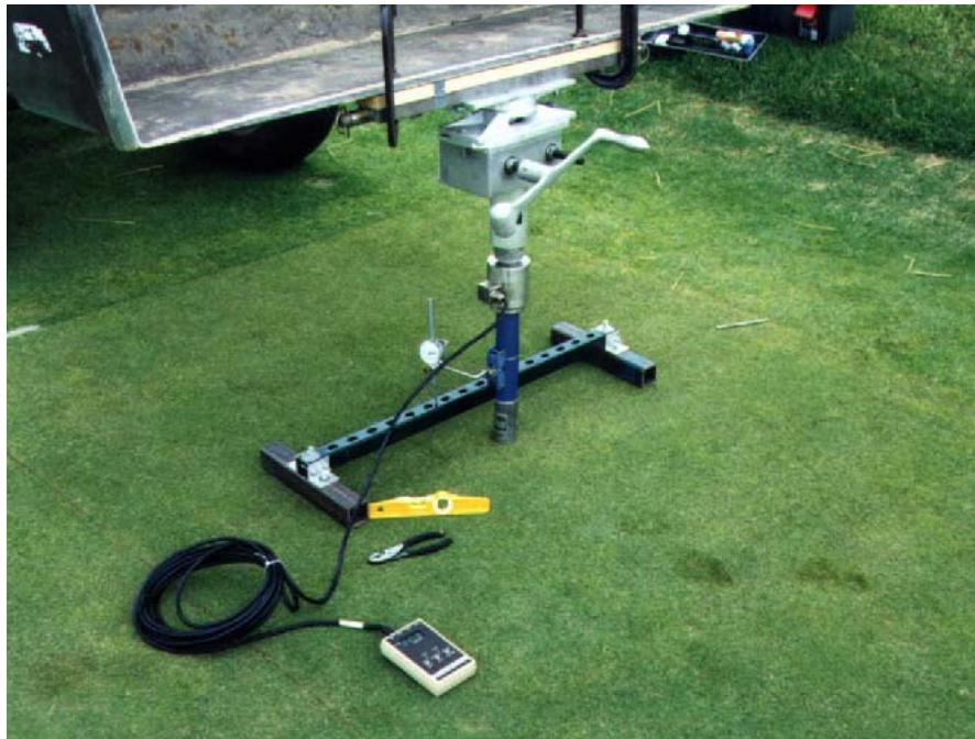
Researchers at Michigan State University used engineering techniques to test the bearing capacity (resistance to surface deformation) of various sands used for putting green rootzones. Although the six experimental sands used in the study all fell with USGA guidelines, the sands varied significantly in their ability to resist deformation from applied pressure.
