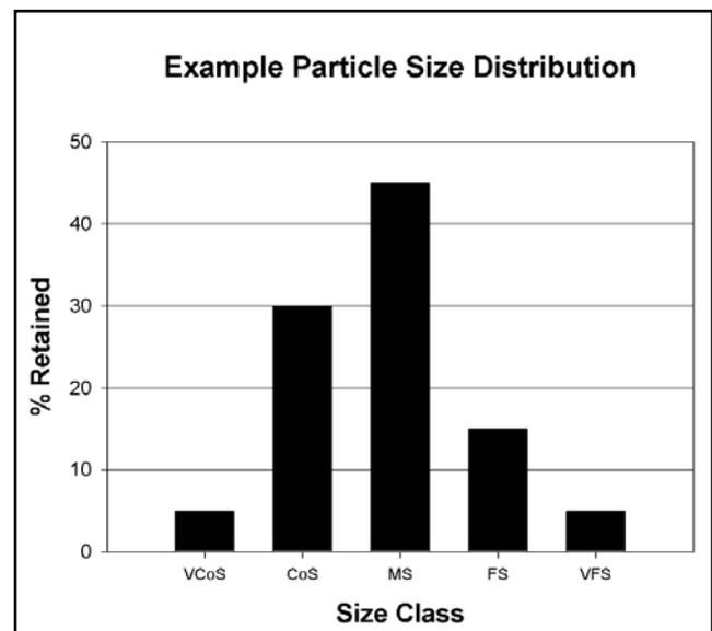
**Figure 1.** Quantifying particle size distribution of sand uses sieve analysis to segregate sand particles according to grain diameters like the example shown above. The United States Department of Agriculture (USDA) defines five classes of sands based on their particle size: very coarse sand (VCoS, 1.0-2.0 mm diameter), coarse sand (CoS, 0.5-1.0 mm diameter), medium sand (MS, 0.25-0.5 mm diameter), fine sand (FS, 0.10-0.25 mm diameter), and very fine sand (VFS, 0.05-0.10 mm diameter).
