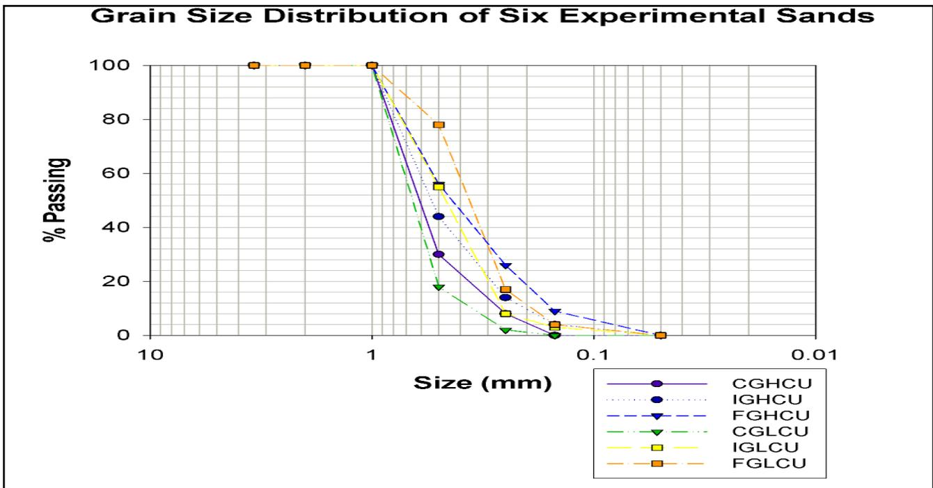
**Figure 7.** Grain size distribution of the six experimental sands used in the Michigan State University study expressed as the percent of the sand sample that passes through various sieve sizes (mm).
