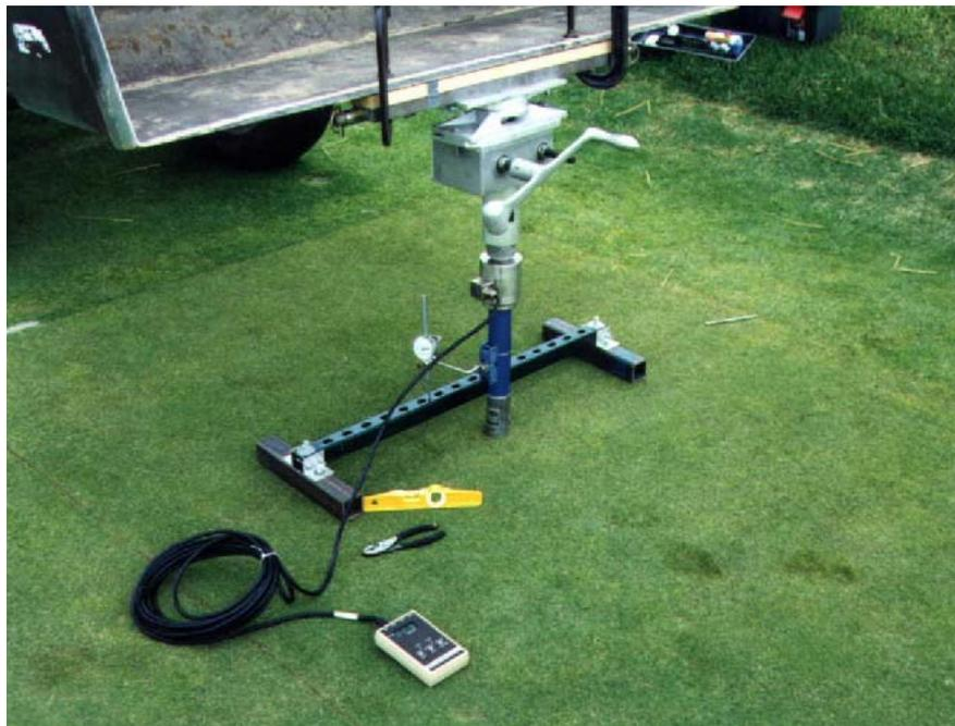
Researchers at Michigan State University used engineering techniques to test the bearing capacity (resistance to surface deformation) of various sands used for putting green rootzones. Although the six experimental sands used in the study all fell with USGA guidelines, the sands varied significantly in their ability to resist deformation from applied pressure.
