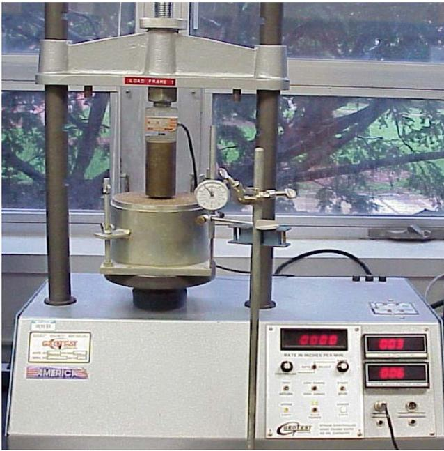
**Figure 3.** A soil's strength against failure under surface compressive load is termed its bearing capacity. This was directly tested in the lab by developing a modified California Bearing Ratio (CBR) testing device.
