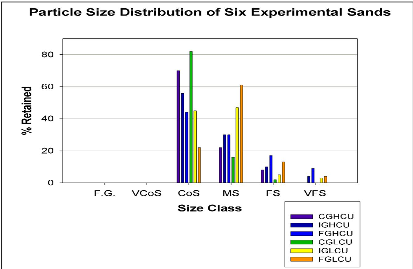
**Figure 6.** Particle size distribution of the six experimental sands used in the Michigan State University study classified by particle size group (i.e., fine gravel, very coarse sand, coarse sand, medium sand, fine sand, and very fine sand)
