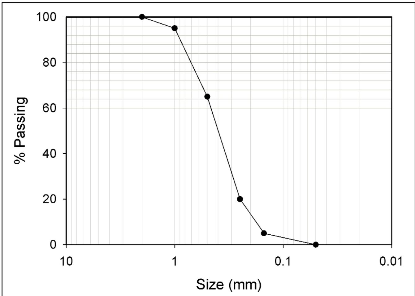
**Figure 2.** Particle size analyses of sands from sieve analyses can also be expressed as a semi-log graph as shown above which plots the percentage of the sand (by weight) that passes through increasingly finer sieve screens against the base-10 log of the grain diameter (mm). Expressing sand this way allows for the determination of the  $D_{50}$  which is the grain diameter value that half the sample is greater than and half the sample is less than.
