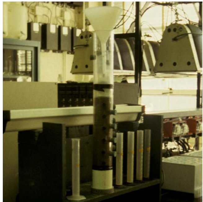
Laboratory procedures were used to evaluate several inorganic amendments compared to sphagnum peat for their ability to affect water retention and percolation in sand-based rootzones.
