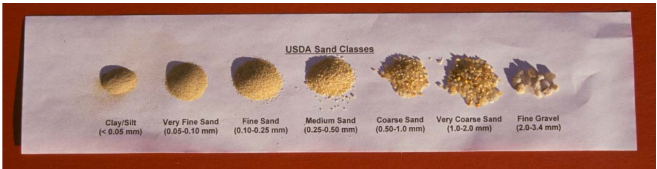
Particle sizes established by the US Department of Agriculture include clay, very fine sand, fine sand, medium sand, coarse sand, very coarse sand, and fine gravel.
