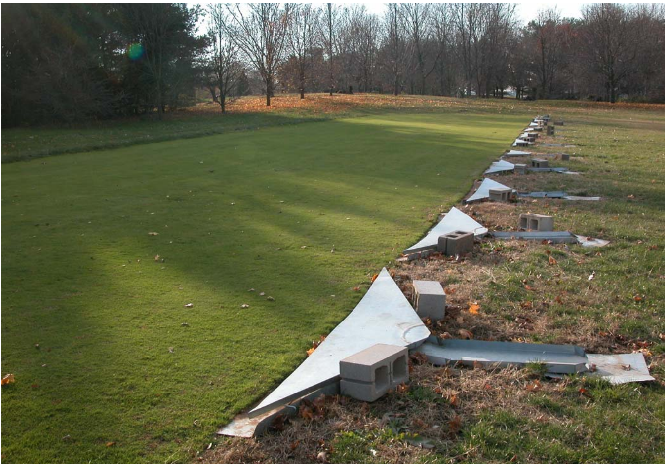
Figure 1. Runoff plots with a 5% slope were constructed at the University of Illinois to study the effects of post-application irrigation and clipping management on runoff of pesticides of varying solubilities.
