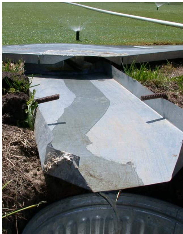
Following pesticide application, irrigation was applied until all plots produced at least 40 liters of runoff.
