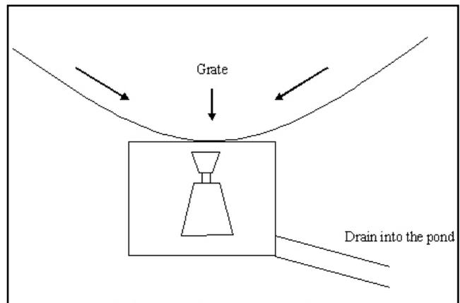
**Figure 7.** The specially designed glass bottles were placed into the fairway drains that eventually drained into the detention pond.
