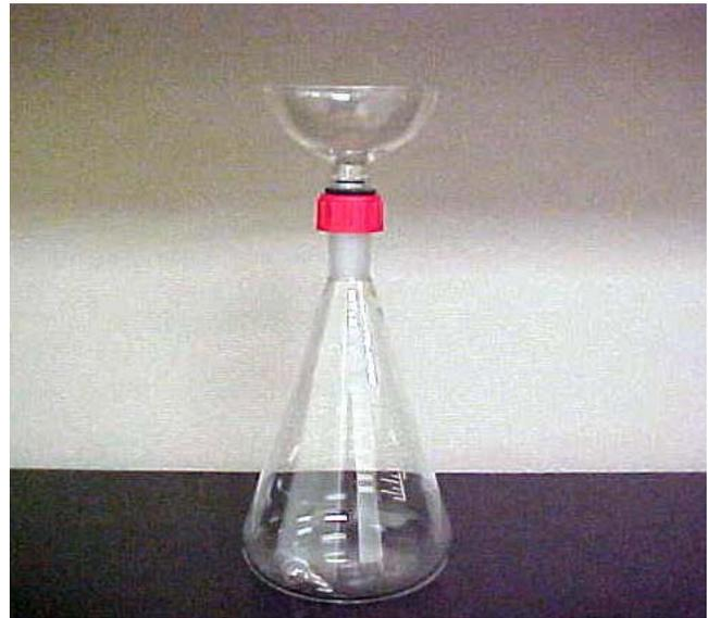
**Figure 6.** To take samples from fairway drains, a glass bottle was developed and used that automatically seals when the bottle is full.
