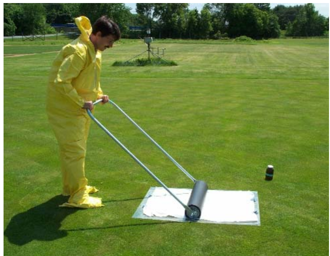
Figure 3. Collecting dislodgeable foliar residues (DFR) with the California roller (CA roller). The 32-lb roller is slowly rolled over a 6 ft 2 cloth 10 times. Pesticide residues transferred to the cloth are considered dislodgeable.
