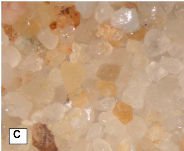
Figure 2. Experiments were initiated in 2003 and 2004 that included treatments of a coarser grade of Black Jack (A), another abrasive aggregate called Amber Jack (B), and Best Sand, an angular topdressing sand (C).
