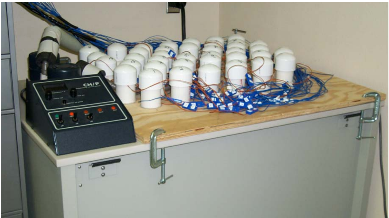
Figure 1. Refrigerated bath modified for use with potted bermudagrass plants. Plants were placed inside plastic tubes glued to a plywood frame
