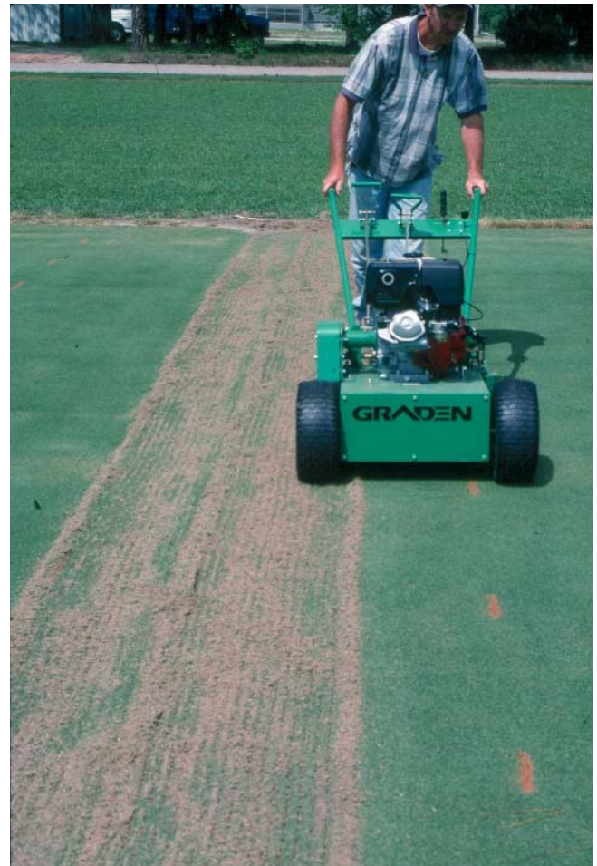
Figure 1. Larry Baldree operating the Graden verticutter to remove thatch in ‘TifEagle’.
