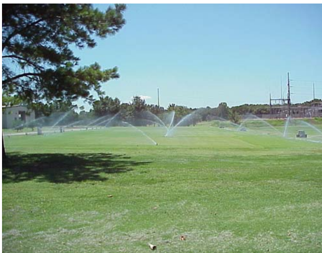
The multiple-barrier rough caused significant delays in time to runoff and lower runoff volume regardless of whether the runoff occurred as a result of irrigation or natural rainfall.
