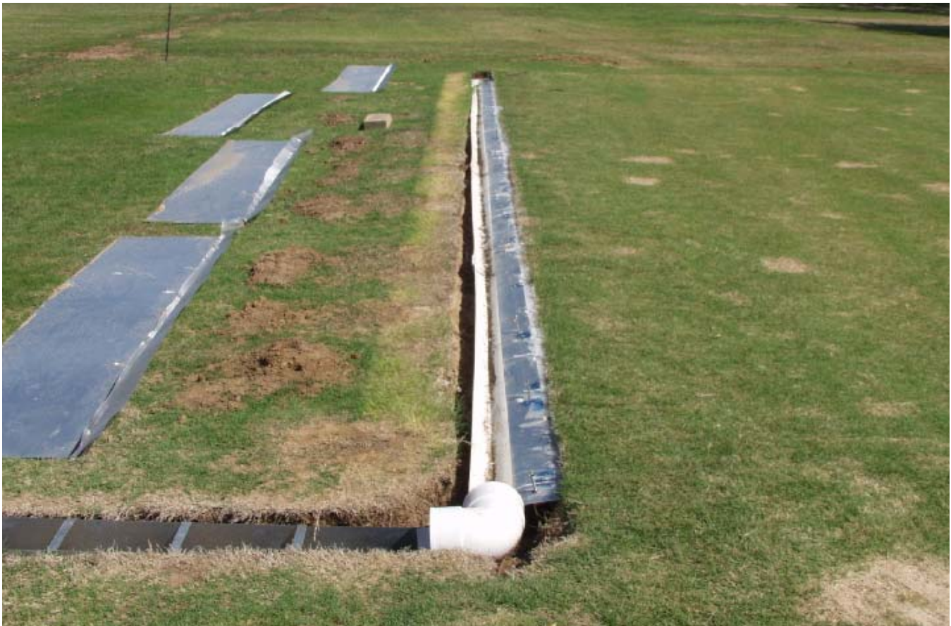
Covered troughs collected runoff water from each plot and channeled it through calibrated Parshall flumes by gravity flow.
