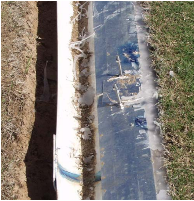
Wax was used to seal the interface of the turfgrass plots with the collection trough to ensure that total runoff was being measured.
