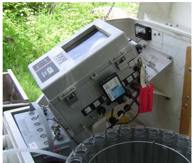
Surface water samples (storm flow and baseflow) from Site 1 and Site 2 were collected throughout the study period using ISCO 6700 automatic collection systems installed on the course.
