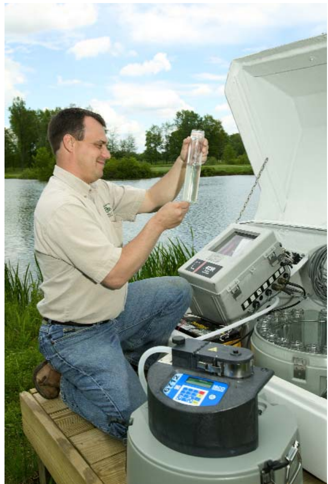
Agricultural engineer Kevin King examines discharge water from a turfgrass system in central Ohio as part of a research program designed to assess how land uses and management affect water quality. This research is funded, in part, by the USGA's Turfgrass and Environmental Research Program.
