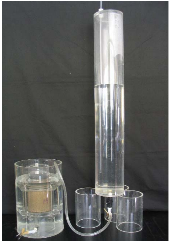
Permeameter for measuring K_{sat} of coarse-textured rooting material.
