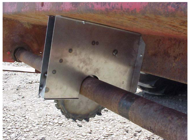
Figure 1. One of four rotating tiller blades mounted on a modified seeder and used to create the 2-inch-wide strip-seeded rows in perennial ryegrass plots and evaluate conversion to seeded 'Riviera' bermudagrass.
