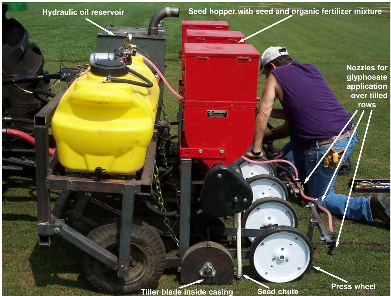
Figure 4. The strip seeder and its components that were used to convert a perennial ryegrass turf to seeded 'Riviera' bermudagrass.
