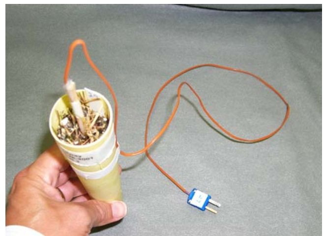
Figure 3. Bermudagrass plant showing thermocouple temperature sensor.
