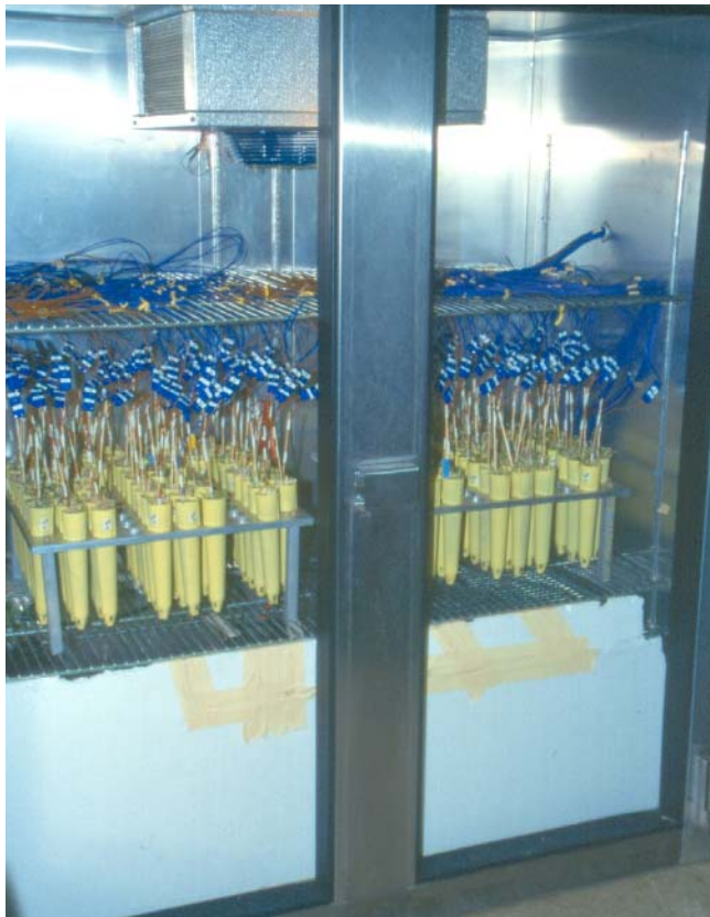
Figure 2. Acclimated plants trimmed of shoots and placed in a programmable freeze chamber for exposure to sub-freezing temperatures.
