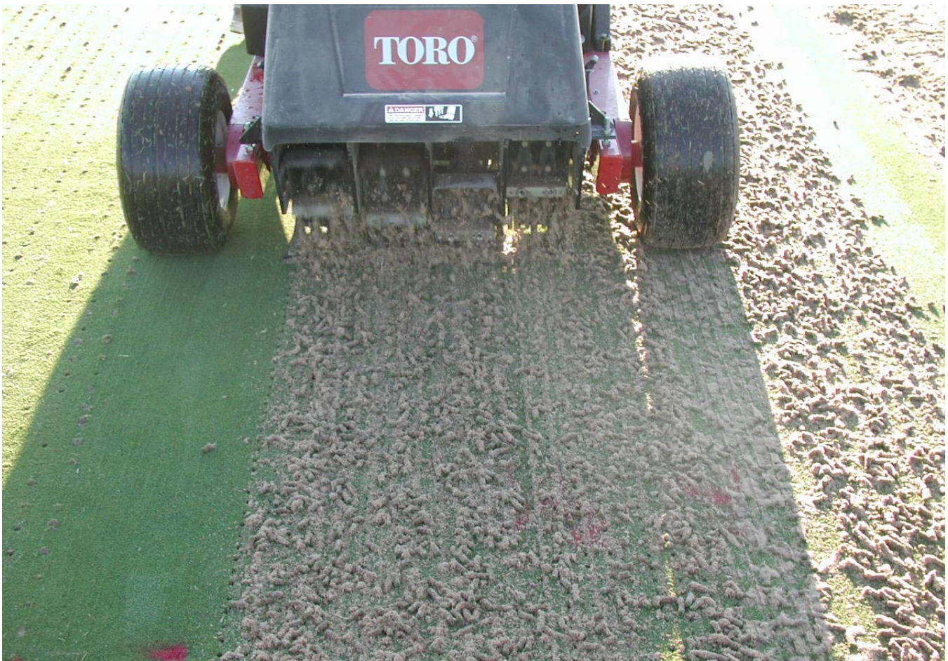
This greens aerator has been retrofitted with tine adapters allowing for a tine spacing of 1.25 x 1.5 inches.
