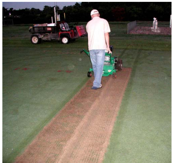
The Graden GS04 verticutter is capable of cutting channels through the surface organic layer of putting green rootzones.
