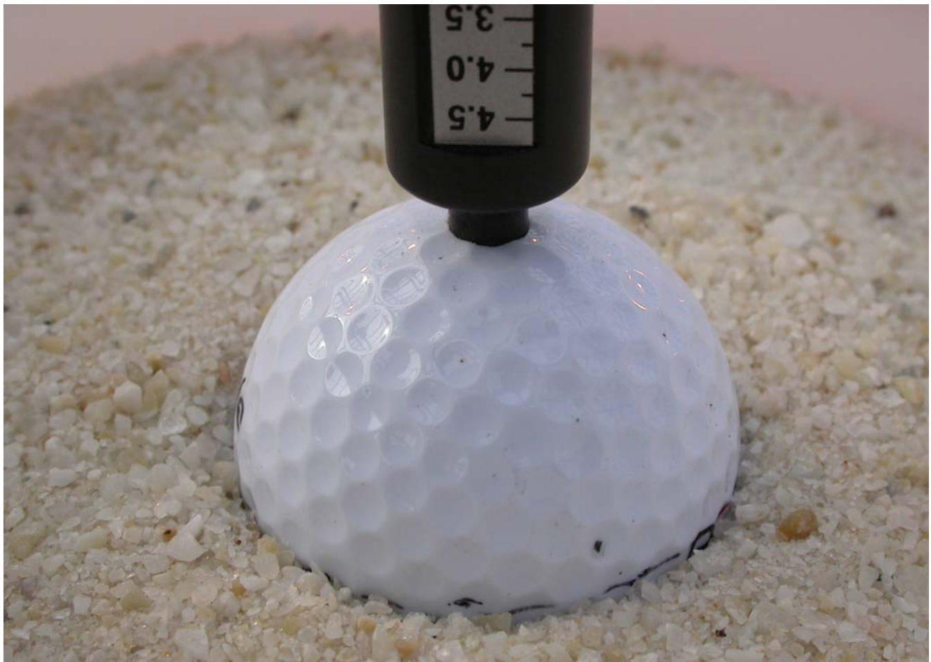
The data most helpful for determining surface hardness is the modified pocket penetrometer test. This test, however, has met with some criticism due to perceived reliability and variability in measurements among users.
