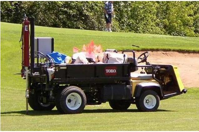
**Figure 2.** Hydraulic probe utilized to collect soil cores from golf course fairways in 2003 and 2004
