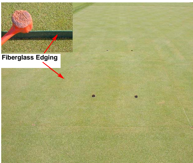
Each plot (1.8 X 2.4 m) was bordered by fiberglass edging set 10-cm deep in soil to minimize lateral movement of water.
