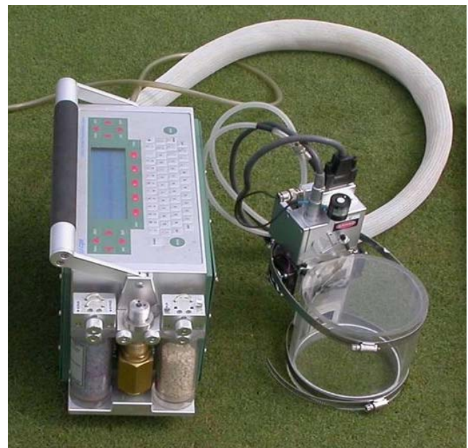
Canopy net photosynthesis (Pn) and whole respiration (Rw) including plant and soil microbe respiration were measured on 2-to 3-week intervals using a portable gas exchange system.
