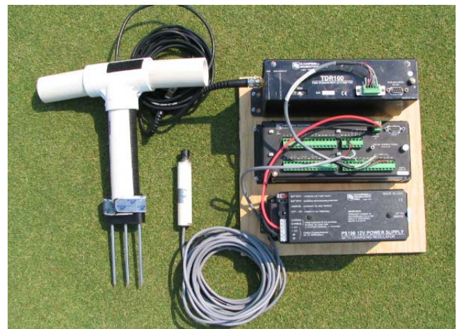
Time-domain reflectometry (TDR) device and datalogger used to measure and store volumetric water content of putting green soils.
