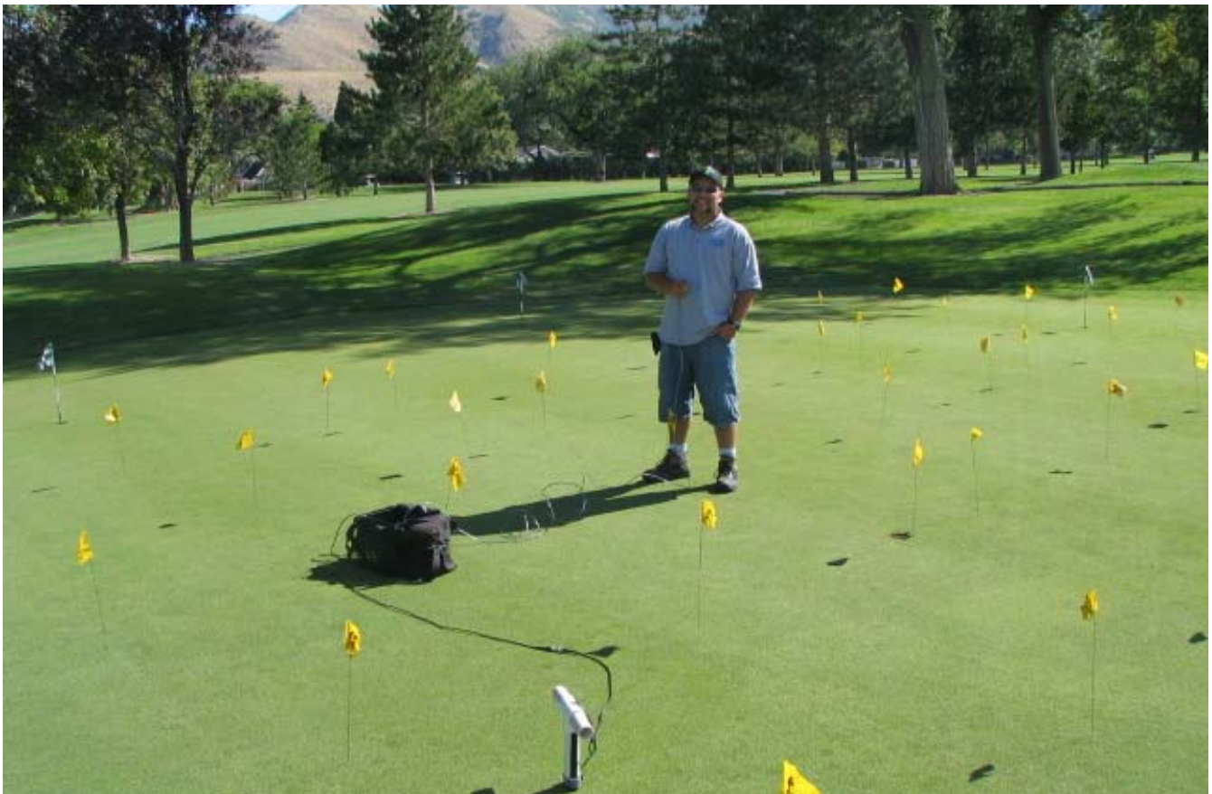
The portable TDR device made measuring rootzone moisture content of individual plots quick and efficient.
