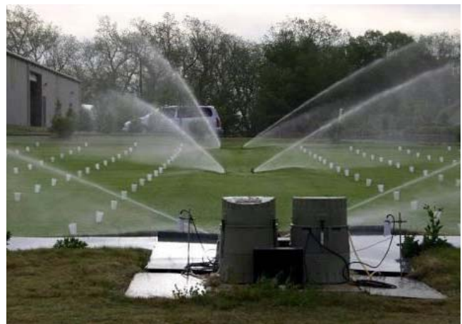
Pesticide and nutrient losses from simulated rainfall did not differ from runoff losses caused by sprinkler irrigation.
