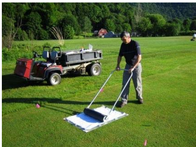
Figure 5. Foliar dislodgeable residues were quantified using the California roller device shown above.
