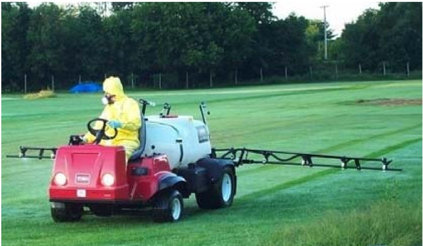
Figure 2. A Toro Multipro 1200 boom sprayer fitted with eleven VisiFlo® flat spray tips (TeeJet® Technologies) was used for all applications.
