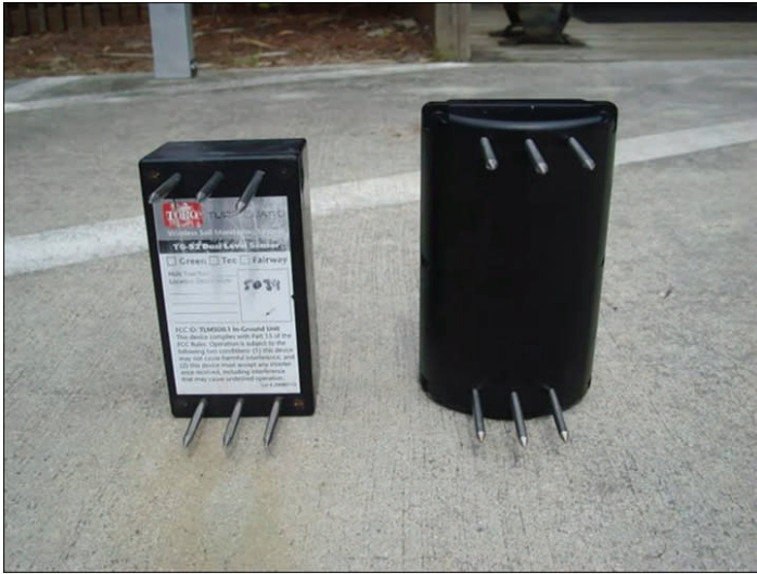
Figure 4. In-ground moisture meters assist in proper irrigation applications.
