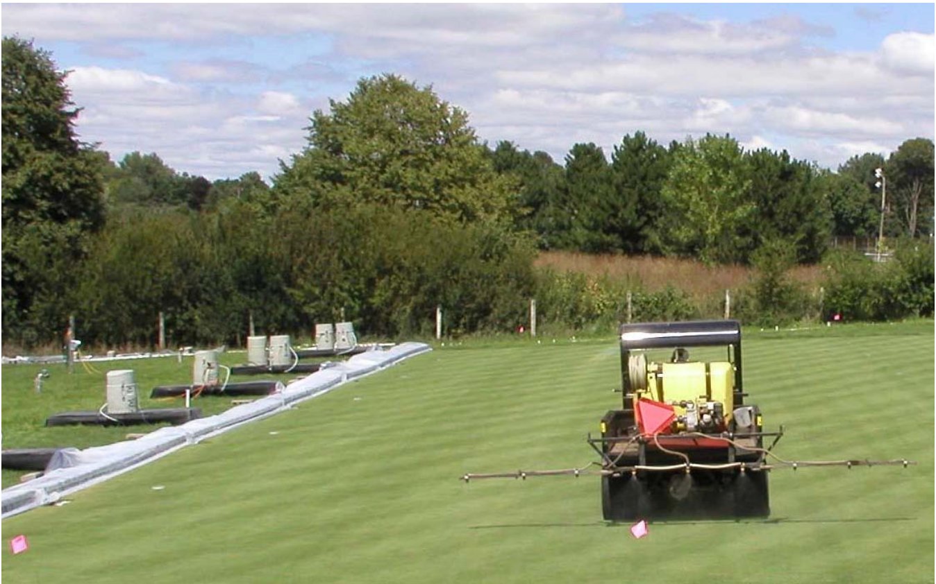
Figure 3. A commercially available insecticide, fungicide, and herbicide were tank mixed and applied at label rates to all plots perpendicular to runoff flow; 63 days and 2 days following core cultivation and 26 ( \pm 13) hours prior to initiation of simulated precipitation and runoff.
