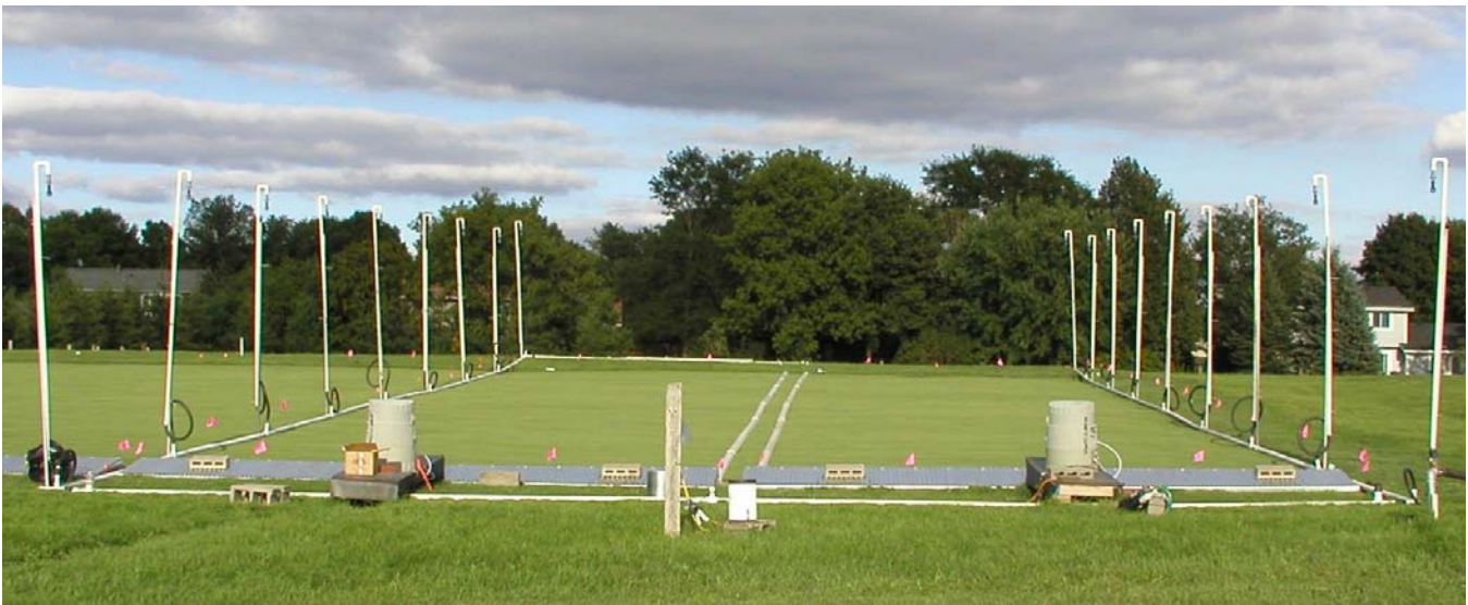
Figure 2. A rainfall simulator delivered precipitation resembling storm intensities recorded in Minnesota. Runoff collection gutters guided runoff from the turf to flumes equipped with automated samplers and flow meters. Gutter covers and flume shields prevented dilution of runoff with precipitation.
