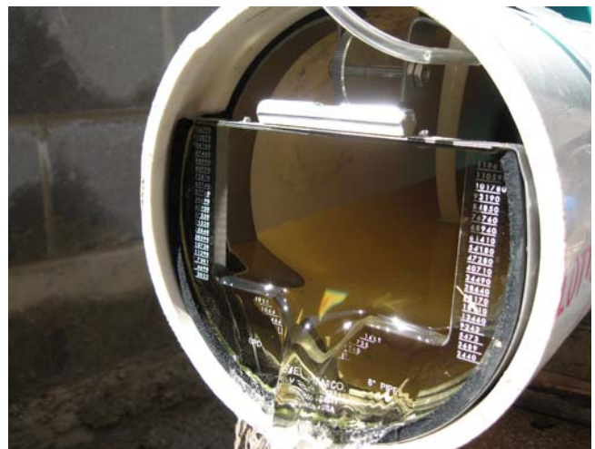
Compound weir insert used to measure the amount of water discharged from a tile.
