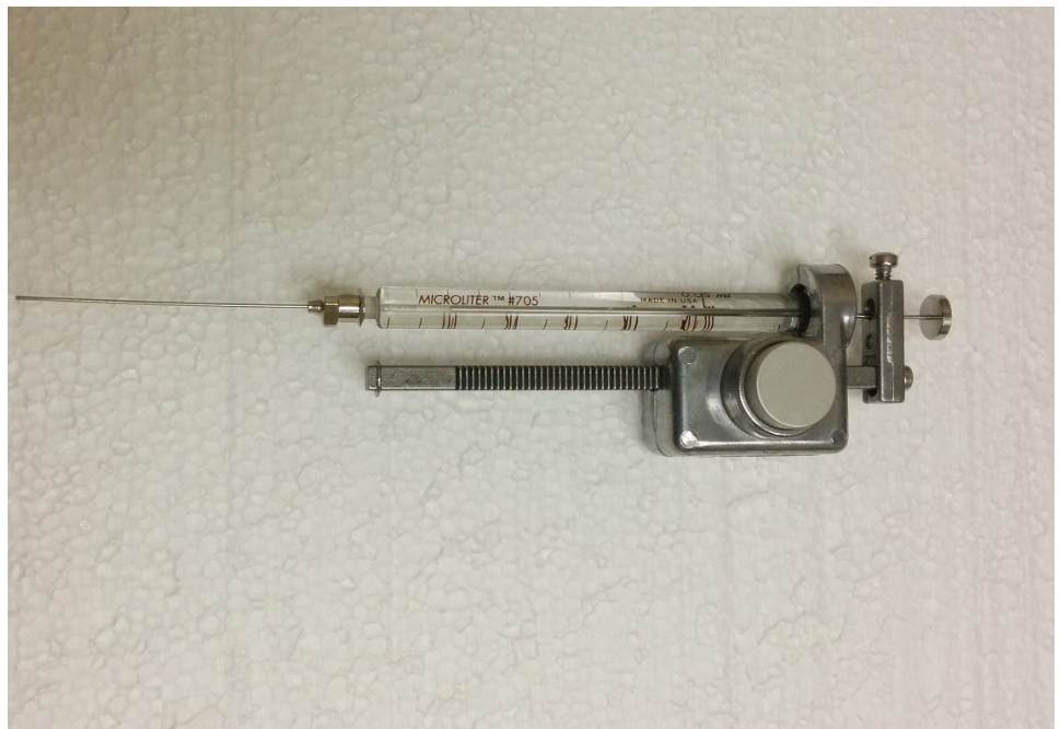
Figure 1. Hamilton microapplicator used for topical application of the insecticide active ingredients (AI).
