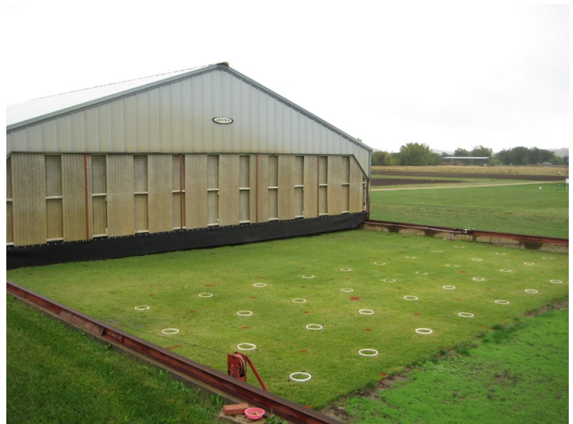
Figure 1. Plots of Meyer zoysiagrass protected from rainfall by an automated rainout shelter. The white rings (one per plot) are PVC collars driven into the ground, on which static chambers are mounted when collecting N_2O flux measurements.
