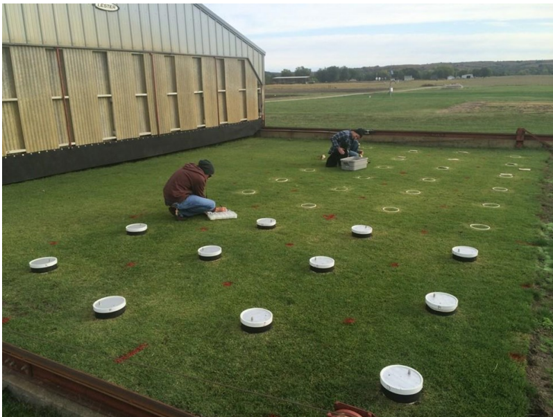
Figure 2: The first measurements of N 2 O emissions were obtained October 6, 2014. In the foreground, static chambers are mounted on the collars during N 2 O flux measurements.
