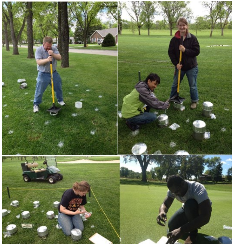
Greenhouse gas sample chambers were tamped into the ground flush with the soil surface. Gas samples were taken a 0, 20, and 40 minutes after the chambers were closed.
