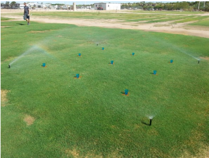
Figure 3. Precipitation tests were run a minimum of five times per plot to accurately determine the precipitation rate of each plot irrigation system.
