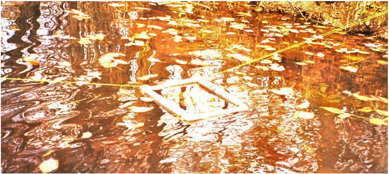
Benthic macroinvertebrate communities of streams adjacent to golf courses were sampled five times in both 1997 and 1998 using artificial leafpack samplers.
