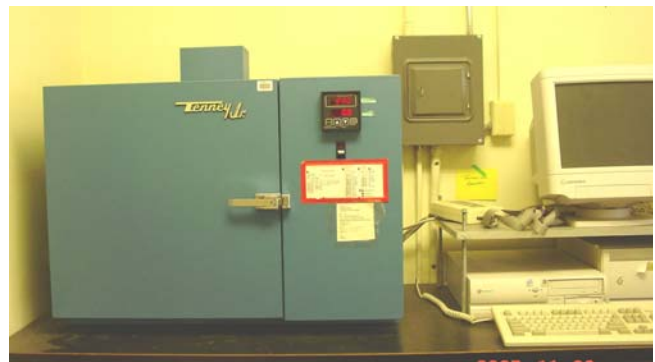
Figure 3. Field grown, acclimated rhizomes of saltgrass were collected and subjected to low temperature treatments ranging from -4^{\circ}\text{C} to -29^{\circ}\text{C} at 2^{\circ}\text{C} intervals using a programmable freezing chamber (shown above). Following freezing treatments, individual rhizomes were planted in a greenhouse and maintained under optimal temperature and moisture conditions to assess survival and regrowth.
