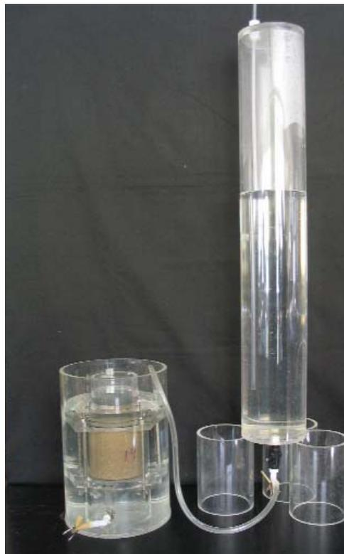
A study conducted by scientists at the University of Southern Illinois was designed to improve the accuracy and repeatability of measuring water movement in prepared putting green rootzone mixes. The study included the creation of a new permeameter (shown above).
