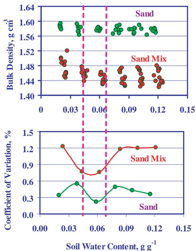
**Figure 5.** Soil-moisture-density curves of sand and sand mix amended with 0.015 g g<sup>-1</sup> of peat moss
