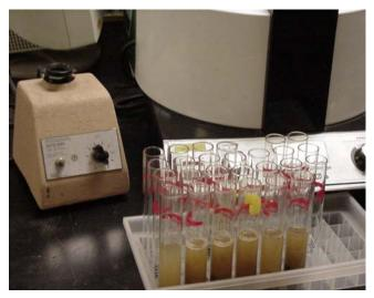
Various extractants were used to best quantify cation exchange capacity (CEC) of calcareous sand because current methods tend to overestimate CEC by dissolving some of the free calcium carbonate contained in calcareous sand.
