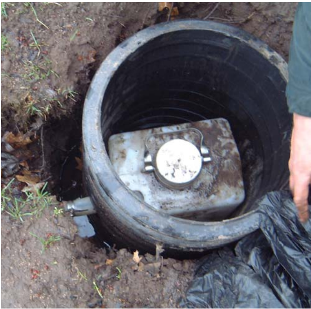
Figure 3. Fairway and buffer strip runoff was collected in Nalgene® containers as water exited from a collection flume at the downslope end of the buffer strips.
