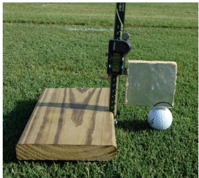
Researchers used a modification of an instrument described by Cella et. al. (1) to measure ball lie.
