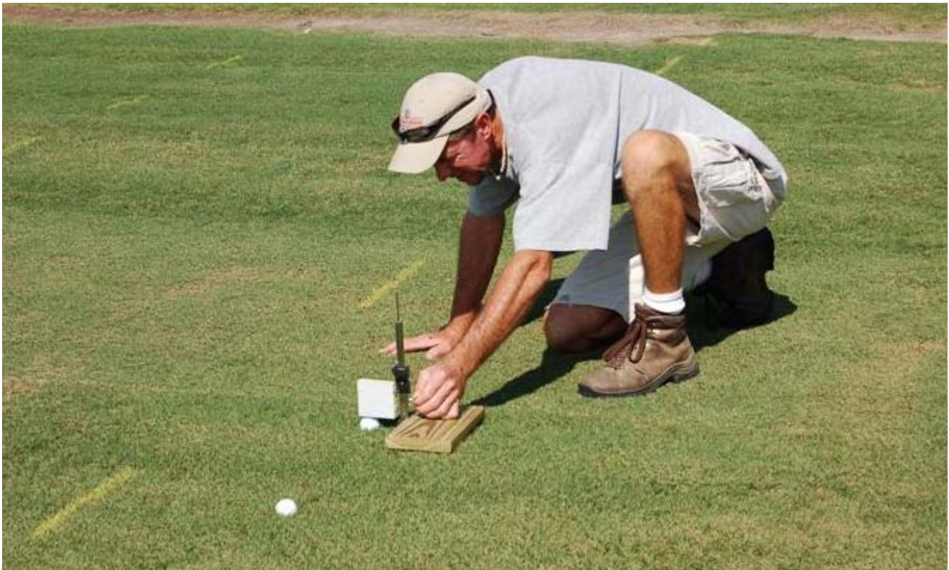
Ball lie measurements were taken by dropping two golf balls into each plot from a height of six feet and then measuring the distance the ball sank into the turf.
