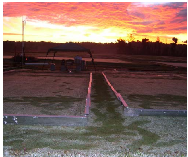
Simulation rainfall events are often conducted at night, or near daybreak, to take advantage of near windless conditions.
