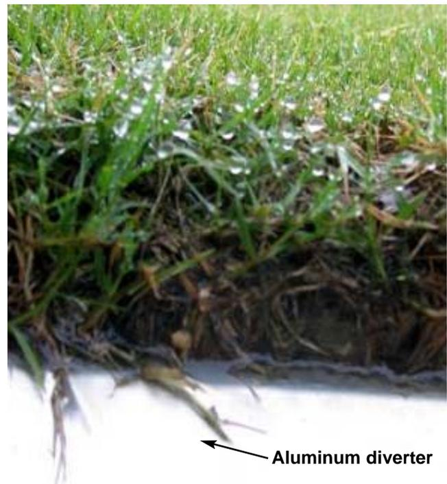
**Figure 3.** Installation of runoff diverter showing overlapping sod on diverter.
