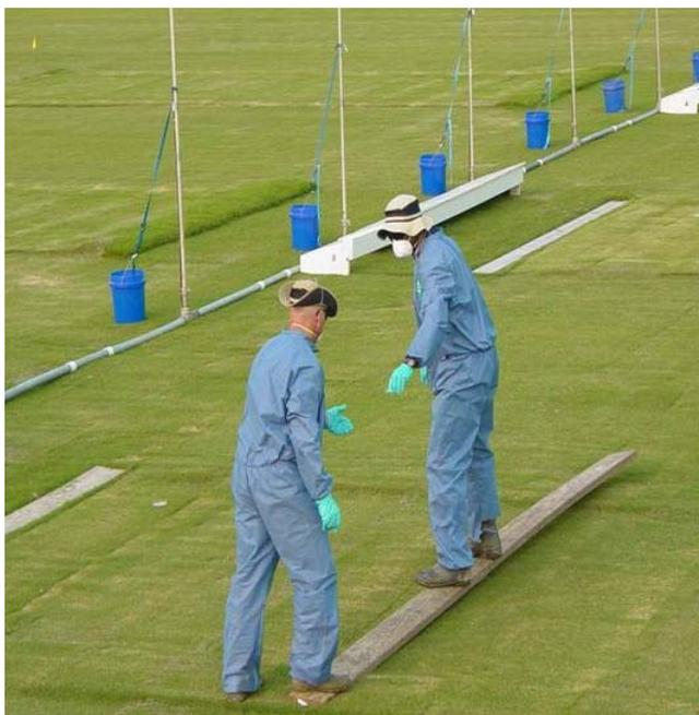
**Figure 6.** Collection of application monitors using catwalk to minimize plot disturbance after pesticide application.
