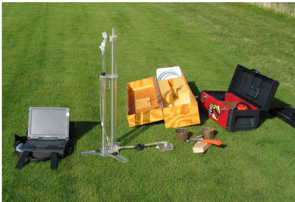
North Dakota State University scientists investigate the use of TDR (time domain reflectometry)-tension infiltrometry methods to predict rootzone water content and movement.
