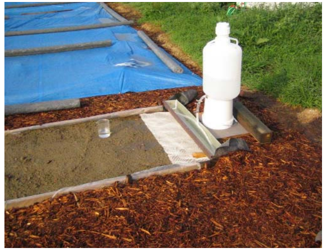
Figure 5. An aluminum manifold with holes drilled at 5-cm intervals allows runoff water to flow evenly onto the top of the VFS
