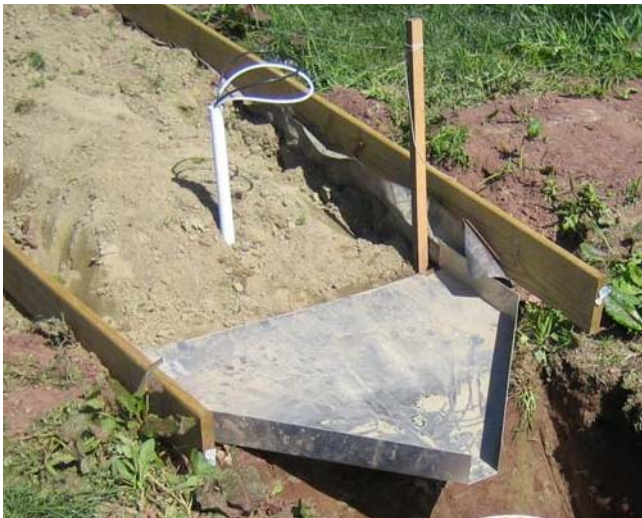
Figure 4. An aluminum sheet collector is located 7.62 cm below the surface of the soil until it exits the soil at the end of the strip and allows the collection of runoff water.
