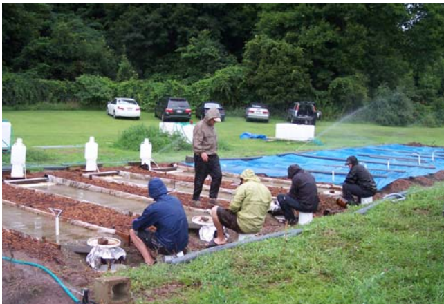
Figure 8. Researchers collect runoff water during a bromide tracer study on VFS prior to plant establishment.
