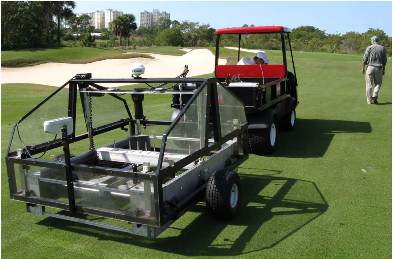
Experimental Salinity Monitoring Device (SMD) conducting salinity mapping of surface salinity, subsurface salinity, and plant NDVI at Old Colliers Golf Club, Naples, FL in May 2009. Data are GPS-labeled and mapping grid is 5 by 10 feet.
