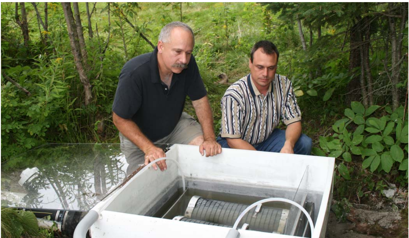
Current research includes investigations involving end-of-tile filters to remove both nutrients and pesticides before drainage water is released to surrounding streams and drainage ditches.
