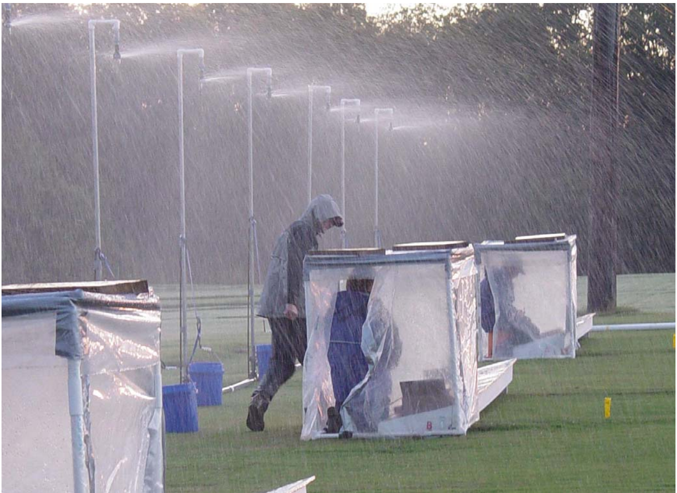
Research at the University of Maryland indicated that greater phosphorus runoff from large-size plots was attributed to mass transport of triple superphosphate granules in large streams of runoff that developed within the these plots during a rainstorm event (5).
