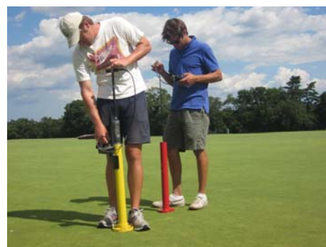
Data collection included surface hardness [Clegg Impact Soil Tester (2.25 and 0.5 kg) and USGA TruFrim].
