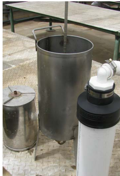
Hydraulic conductivity will be measured using an automated falling head permeameter.
