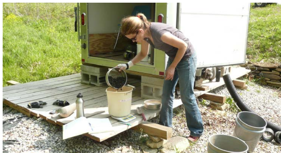
Each tile was filled with 28.5 kg of steel slag that was previously removed of fines with a U.S. Standard Mesh #16, 18 mm sieve.
