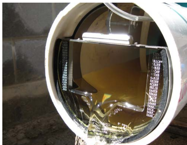
Compound weir insert used to measure the amount of water discharged from a tile.
