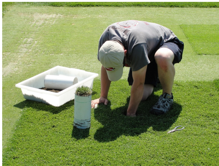
Figure 1. Installation of mini-lysimeters into tall grass perennial ryegrass plots.
