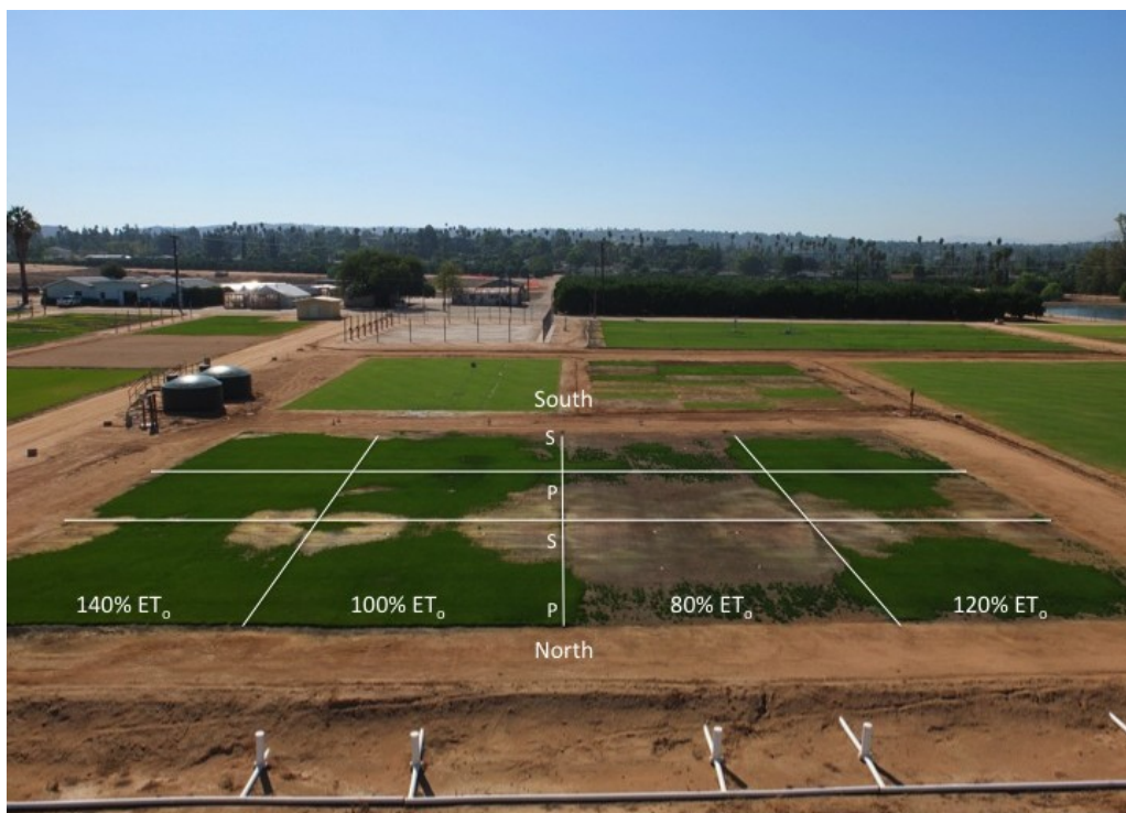
Figure 1. Turfgrass salinity research area in October 2012 in Riverside, CA. Alternating irrigation lines are fed by potable (P) or saline (S) water. Two 5,000-gallon tanks are used to store and deliver saline irrigation water. In the perpendicular direction, the area is divided into four irrigation zones, ranging from replacement of 80 to 140% ET_o . Two subsurface drain lines bisect each of the irrigation zones with outlets for collection of leachate. Twelve 30-ft x 30-ft plots represent a continuous distribution of saline and potable water at a given irrigation regime.
