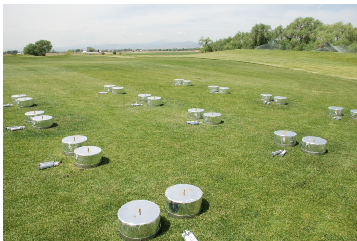
Figure 3. For trace gas sampling, the vented chambers were installed onto the PVC anchors. Air samples were removed from each chamber.
