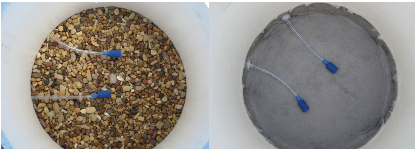
Figure 3. Test greens constructed in 14-inch PVC pipe with either gravel or geotextile atop AirDrain as the drainage layers. Both types of test greens contained a pair of porous cups connected to plastic tubing that formed manometer–tensiometers to allow measurement of water pressure or tension at the root zone–drainage layer interface.
