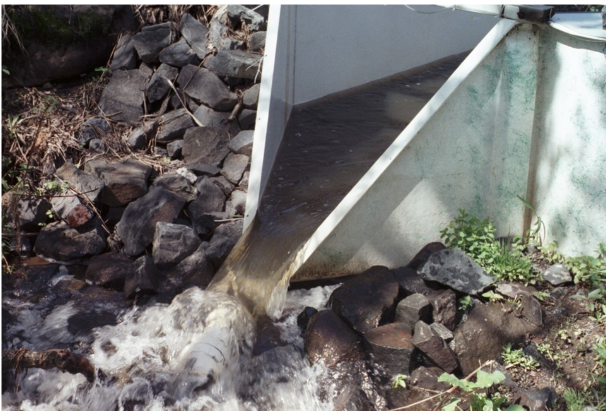
Figure 2. Installed H-flume at Northland Country Club (NCC) in Duluth, MN.
