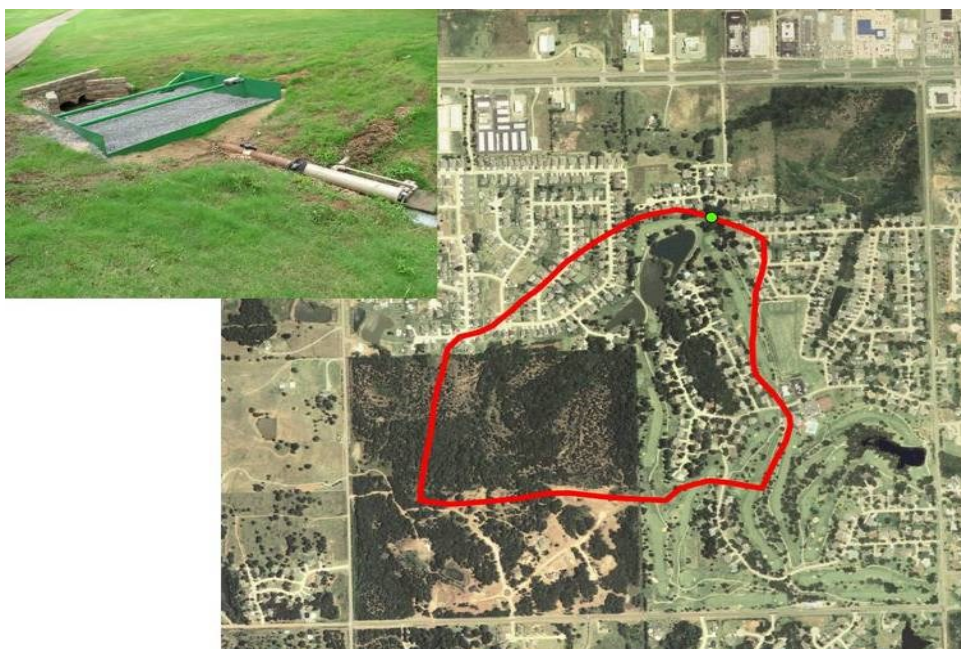
Figure 1. Phosphorus removal structure located at Stillwater Country Club. The unit treats runoff water at the outlet of a 150 acre watershed.
