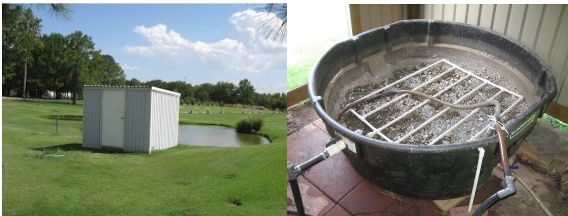
Figure 4. Pilot scale P pond filter. Water from the pond is continuously pumped into the bed of PSMs contained in building. The filtered water drains back into the pond.
