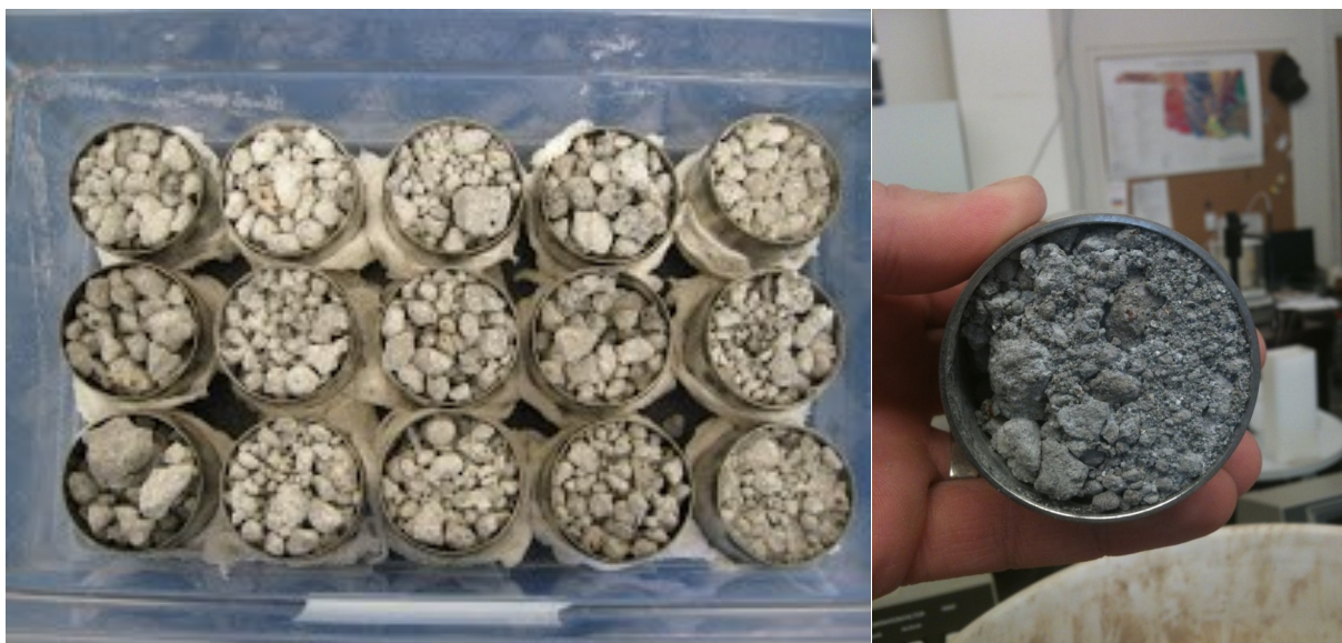
Figure 2. Various sized steel slag fractions tested for hydraulic conductivity. Picture on the right show the non-sieved slag after the test. Note the crusting and cementing of particles which resulted in a decrease in hydraulic conductivity.
